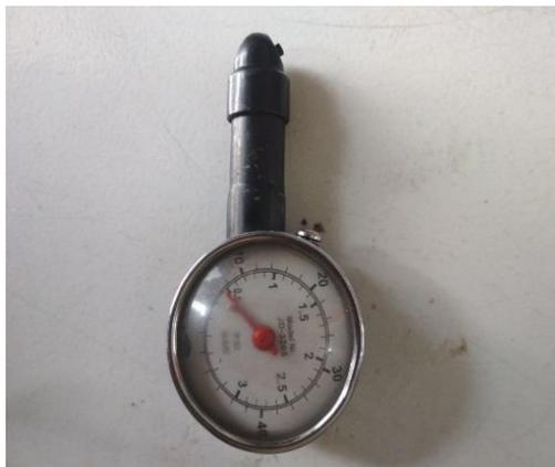
**Gambar 3.11** Tire pressure meter
