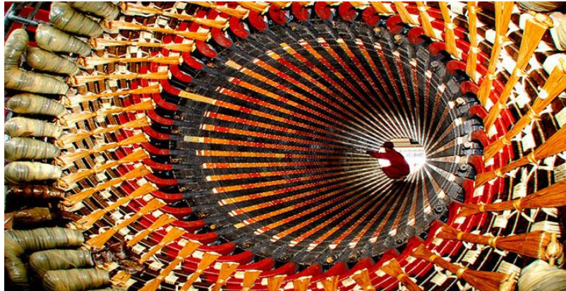
Gambar 2.2. Stator generator sinkron
