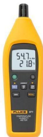
Gambar 3. 12 *Fluke 971 Temperature Humidity Meter* [17].
