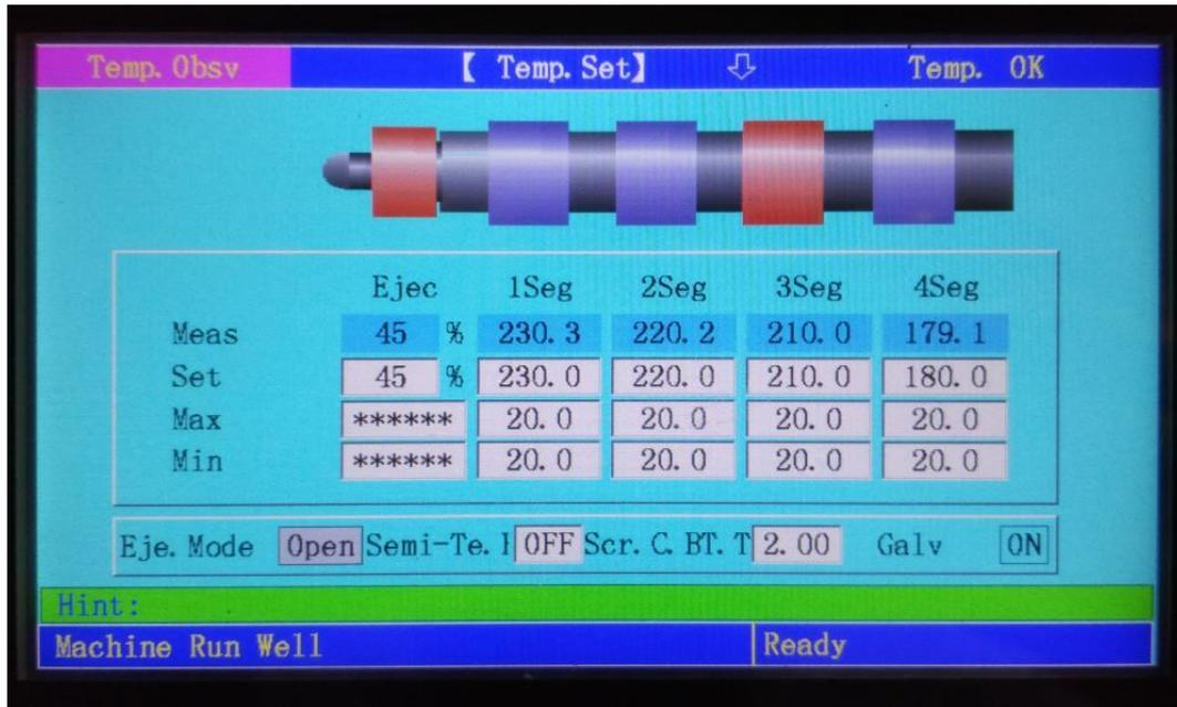
**Gambar 3.20.** Panel Parameter Temperatur Barrel
