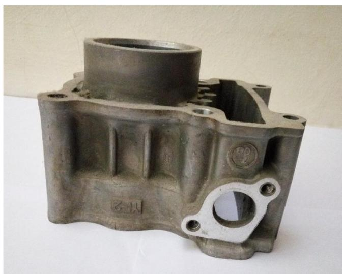
Gambar 3. 4 Blok Silinder Yamaha Jupiter Mx
