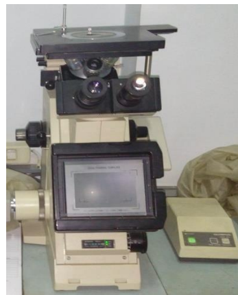
Gambar 3.13 Alat uji foto mikro merek OLYMPUS model PME3-111B/-312B
