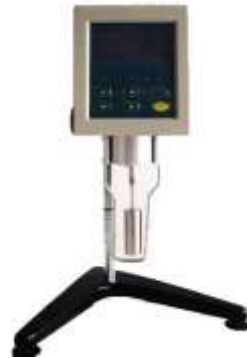
Gambar 3.1 Alat Viscometer NDJ 8S
