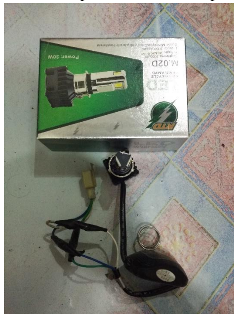
Gambar 3.3 Lampu utama LED RTD ( AC & DC 9- 18 V, power 30 W)
