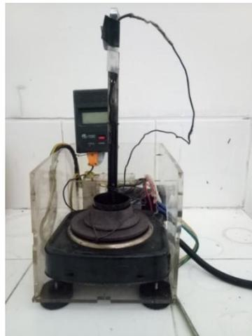
Gambar 3.19. Alat Uji *Flash Point*
