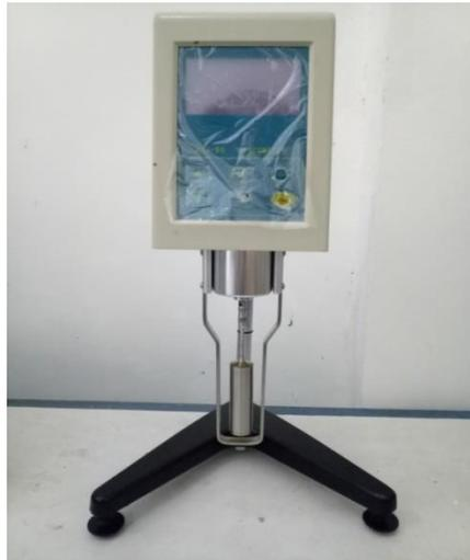
Gambar 3.17. *Viscometer NDJ 8s*
