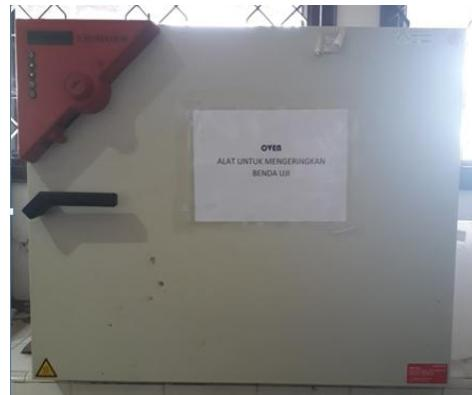
Gambar 1 Oven suhu maksimal  $220^{\circ}\text{C}$
