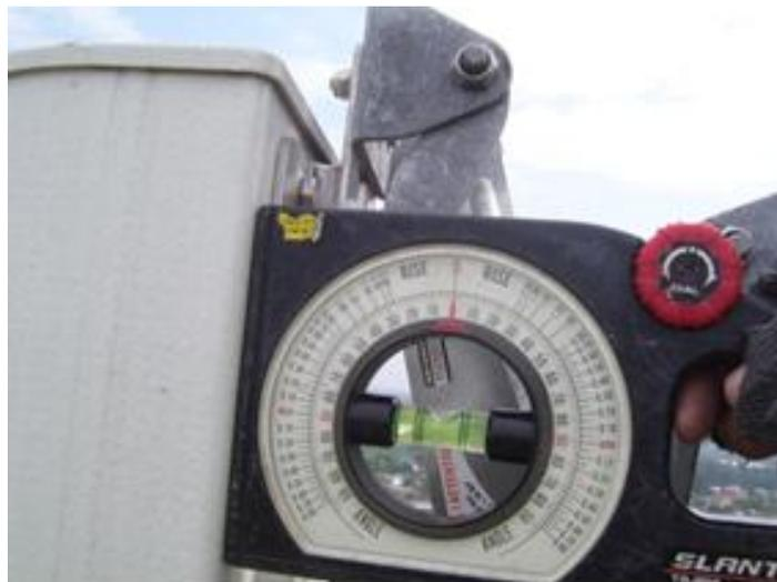
Gambar 2.6. Alat ukur *tilt meter*
