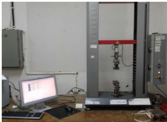
Gambar 3.3 Universal Testing Machine (UTM)
