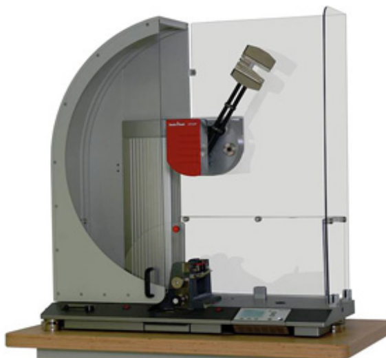
Gambar 3.5 Alat uji impak model charpy
