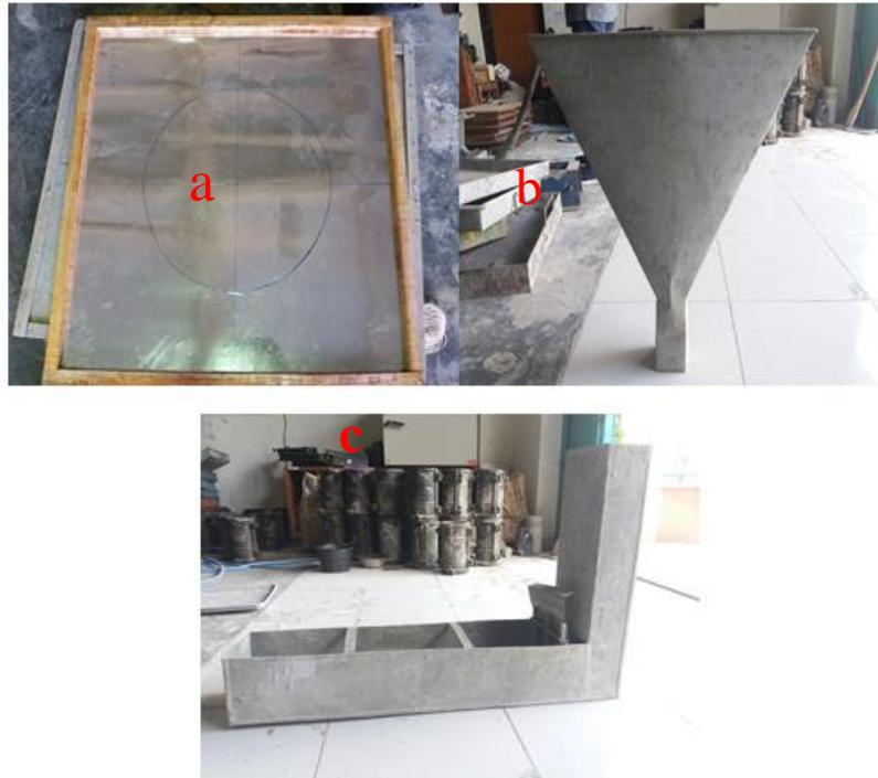
Gambar 3.20 Alat pengujian: (a) Meja Sebar (T50), (b) V-Funnel, (c) L-Box
