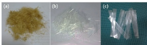
Fig. 1: Chopped kenaf fibers (a) and E-glass fibers (b), and cut PP sheets (c) used in the hybrid composite fabrication.
