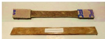
Fig. 2: Profile of the hybrid composite sheet (the bottom) and the tensile test specimen (the top).
