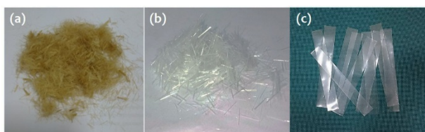
Fig. 1: Chopped kenaf fibers (a) and E-glass fibers (b), and cut PP sheets (c) used in the hybrid composite fabrication.
