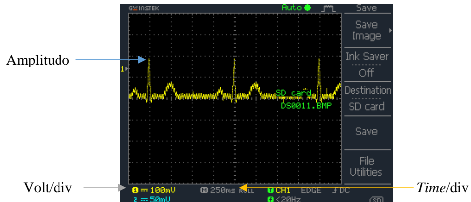
Gambar 4. 5 Output instrument amplifier lead II amplitudo 1 mV
