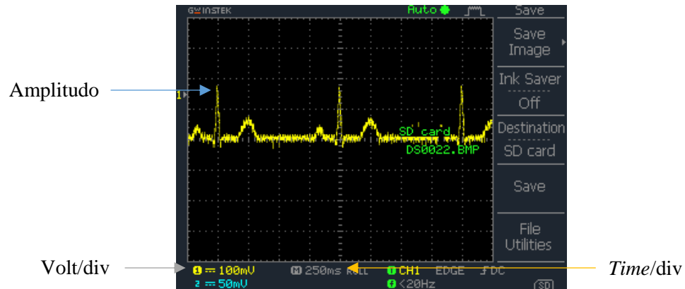
Gambar 4. 9 Output instrument amplifier lead III amplitudo 1,5 mV
