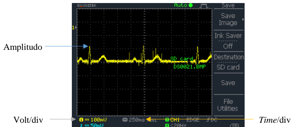
Gambar 4. 8 Output instrument amplifier lead III amplitudo 1 mV
