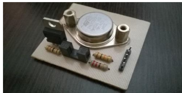
Gambar 3.9 Rangkaian Fisik Driver Motor DC
