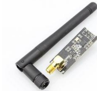
Gambar 2.4 Modul nRF24L01 +PA+ LNA + Antena SMA
