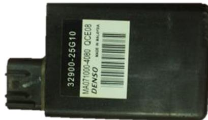
**Gambar 2.4** CDI (*Capasitor Discharge Ignition*)
