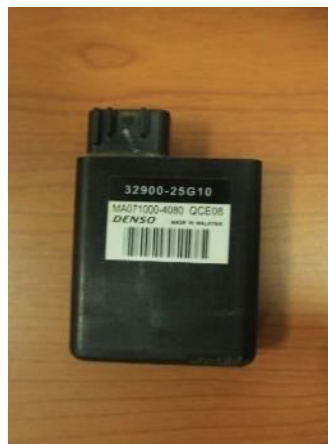
Gambar 3.2. CDI Standar Suzuki Satria FU 150 cc
