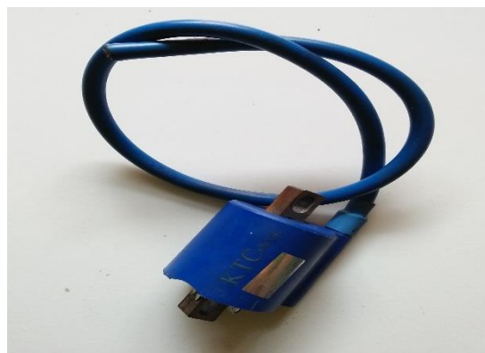
Gambar 3.5. Koil Racing KTC
