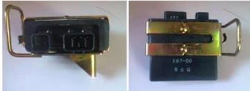
**Gambar 2.7** CDI ( Capasitor Discharge Ignition )
