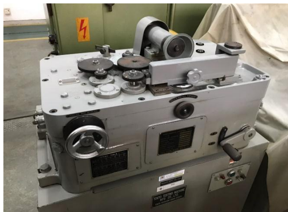
Gambar 3.14 Alat Uji Keausan (Riken-Ogoshi Universal Wear)
