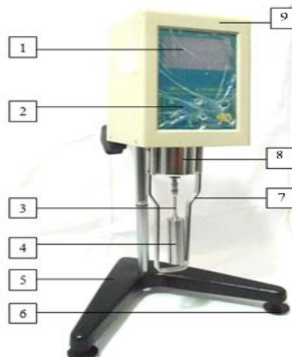
Gambar 3.21 Bagian-bagian viscometer NDJ 8S.
