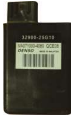
Gambar 3.2. CDI Standar Suzuki Satria FU 150 cc
