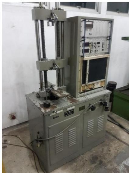
Gambar 3.20 Mesin uji *bending* Torse Universal Testing Machine
