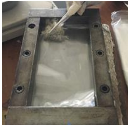
Gambar 3.46 Proses Hand - Lay -Up
