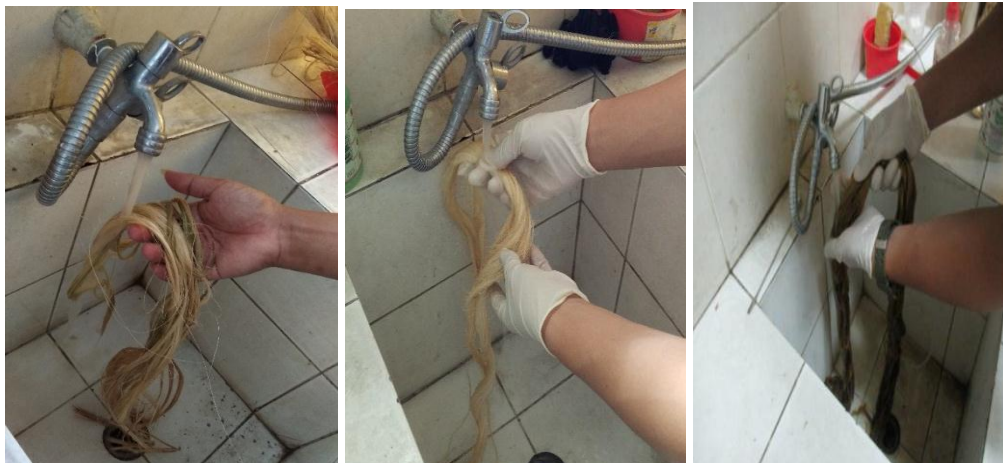
Gambar 3.27 Proses Pencucian Serat Alam
