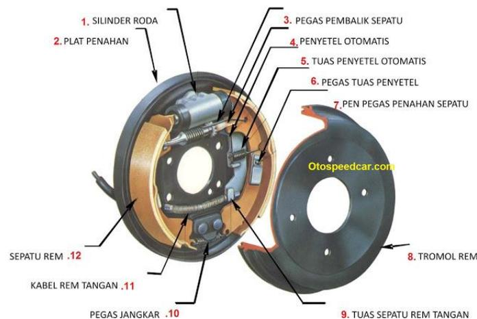
**Gambar 2.1** rem *drum*/tromol
