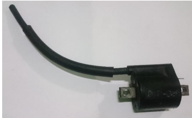
Gambar 3.19 Koil standar Yamaha Jupiter Z 110 cc
