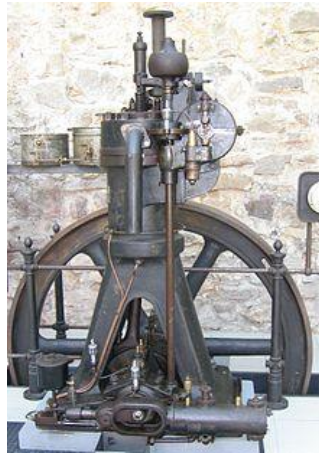
Gambar 2.1. Mesin diesel silinder tunggal Rudolf Diesel (Budiman, 2017)
