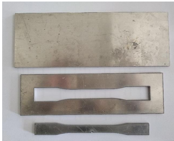
Gambar 3. 10 Molding ukuran ASTM D638-01
