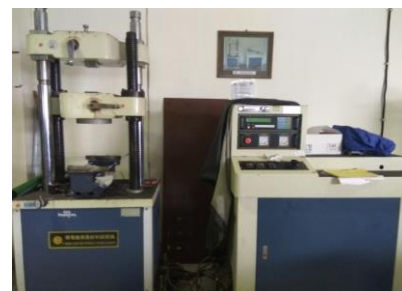
Gambar 1 Universal machine test Pengujian kuat lentur beton SCC
