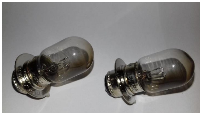
Gambar 3.2 Lampu standar pabrik (12 volt, power 25 watt)
