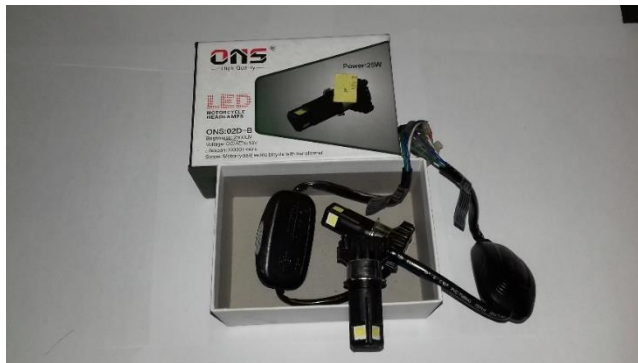
Gambar 3.1 Lampu LED ONS 3 sisi (AC dan DC 9-18 volt, power 25 watt)
