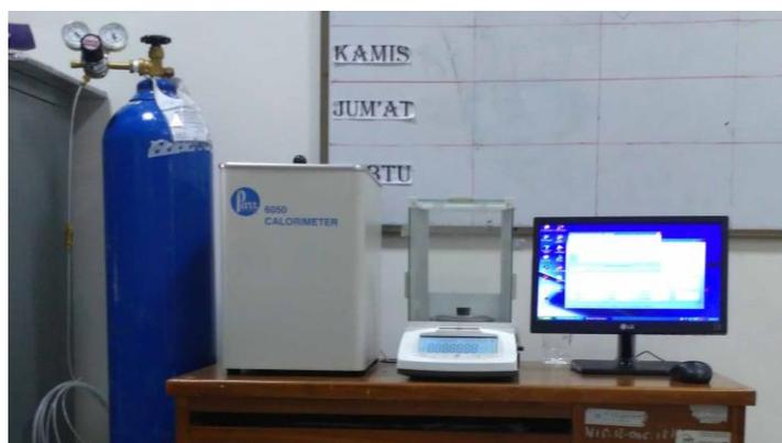
Gambar 3.13. Alat bom kalorimeter
