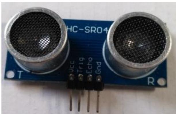
Gambar 2.2 Sensor Ultrasonik HC – SR04
