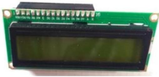
Gambar 2.8 LCD (*Liquid Crystal Display*)
