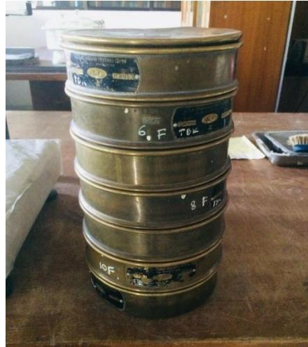
Gambar 3. Saringan ASTM
