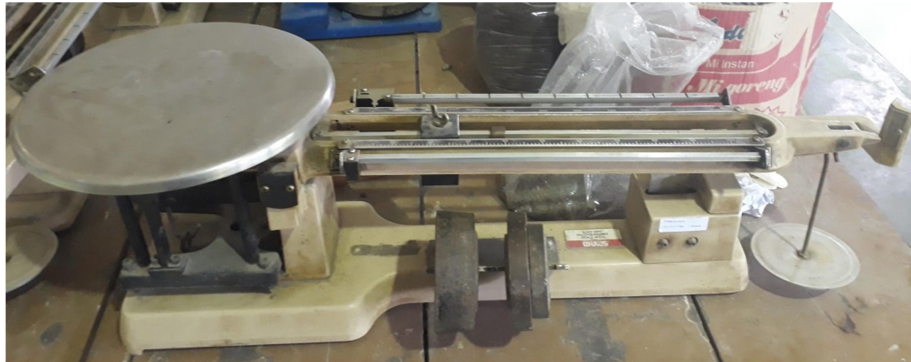
Gambar 3. 3 Neraca ohaus ketelitian 5 gram
