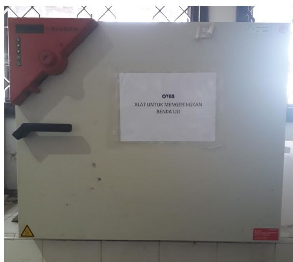
Gambar 3. 1 Oven suhu maksimal 220 0 C
