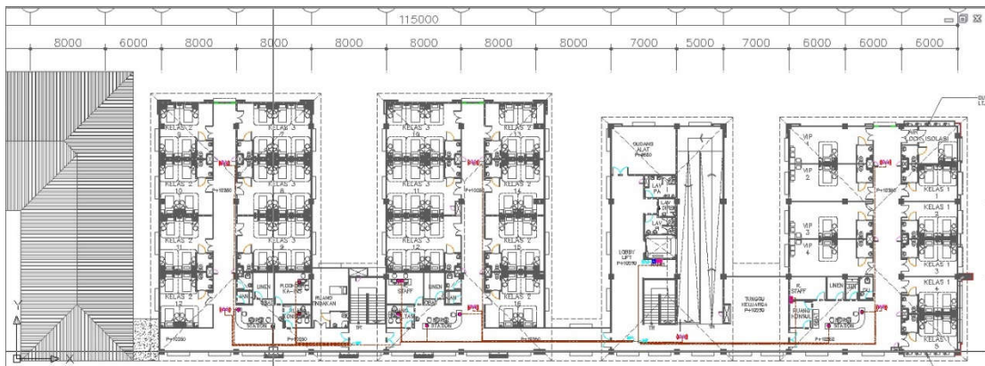
Gambar 4.11 Denah Perancangan WiFi AP Lantai 3
