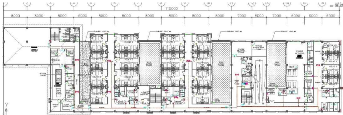
Gambar 4.9 Denah Perancangan WiFi AP Lantai 2
