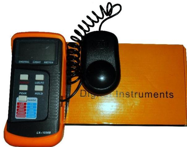
Gambar 3.7 Digital Lux Meter
