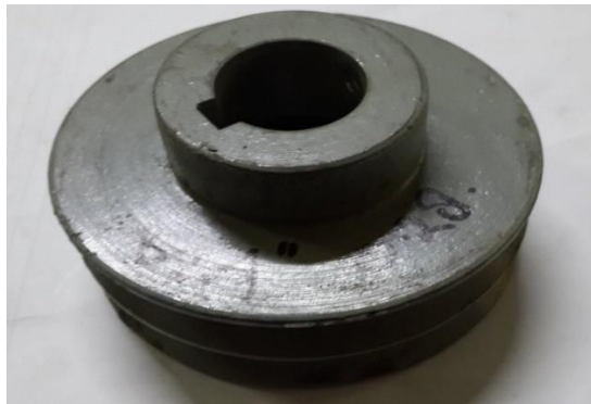
Gambar 4 Pulley diameter 10 cm
