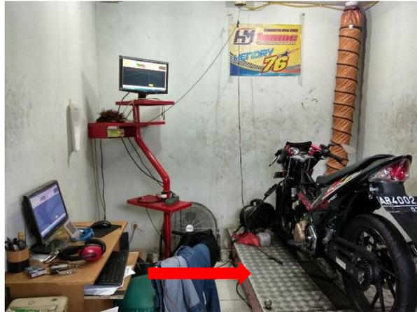
**Gambar 3.8** *Dynamometer*
