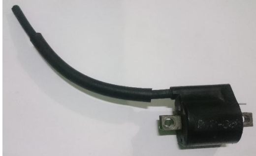
Gambar 3.16 Koil standar Yamaha Jupiter z 110 cc
