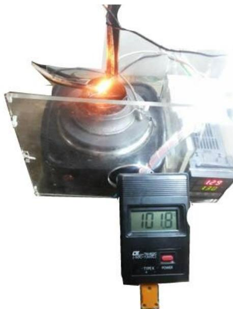
**Gambar 3.13** Alat uji *flash point*
