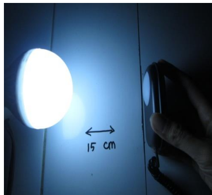
(c) Pengukuran LUX lampu LED BULB
