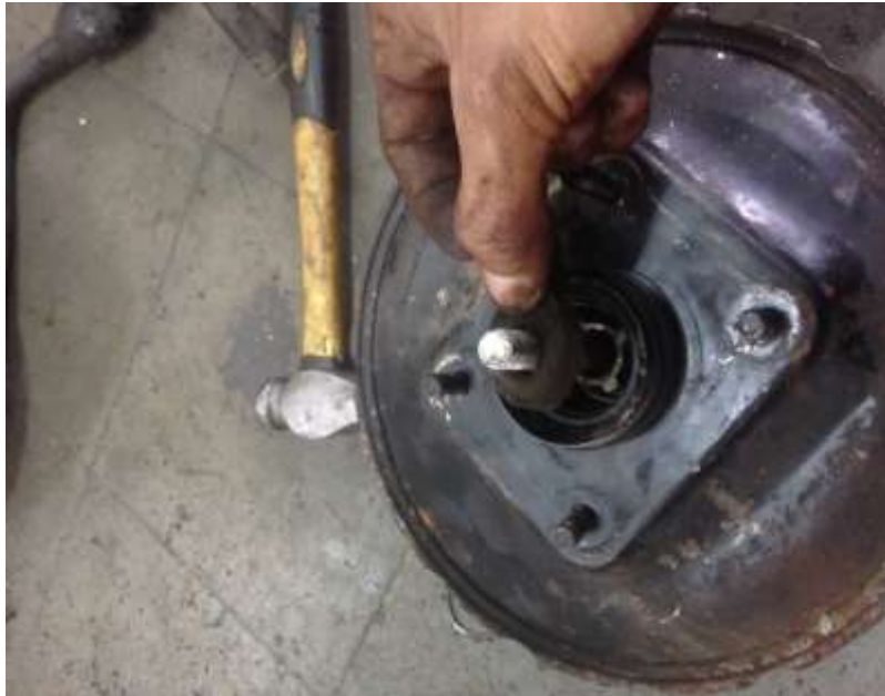
Gambar 3.5 Pembongkaran Booster Housing
