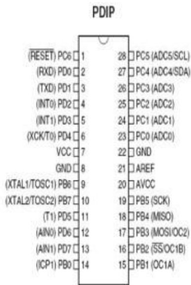
Gambar 2.3 Pin-out ATmega 8 [6].
