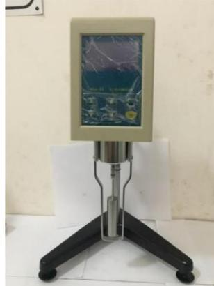
Gambar 3.12 Viskometer
