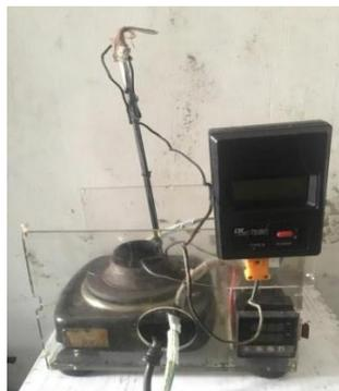
Gambar 3.15 Alat Uji *Flash Point*
