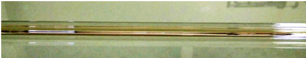
Gambar 3.3 Test Section (pipa diameter 1,6 mm )
