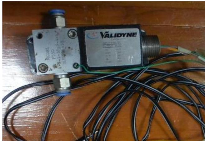
Gambar 3.15 *Pressure transducer*
