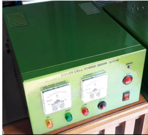
Gambar 2.8 Solar Charger Controller
