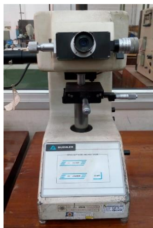
Gambar 3.22 Micro hardness tester type HVL
