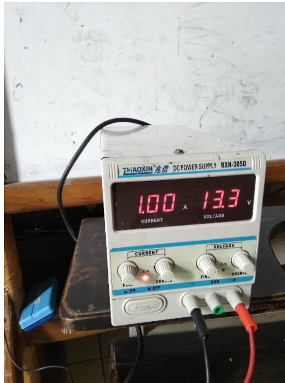
Gambar 3.6 Power Supply type Thaoxin RXN 305D
